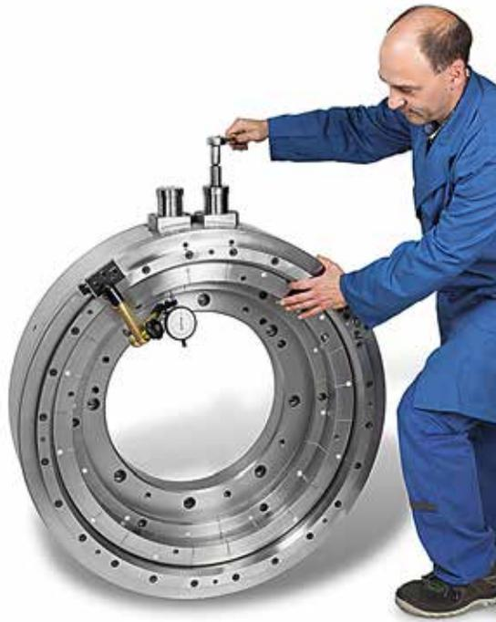
A MyTEC technician checks the runout of a large clamping tool.
