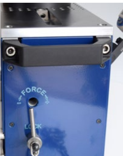
Lever to infinitely adjust the measuring force
