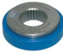
Control master to monitor measuring instruments
