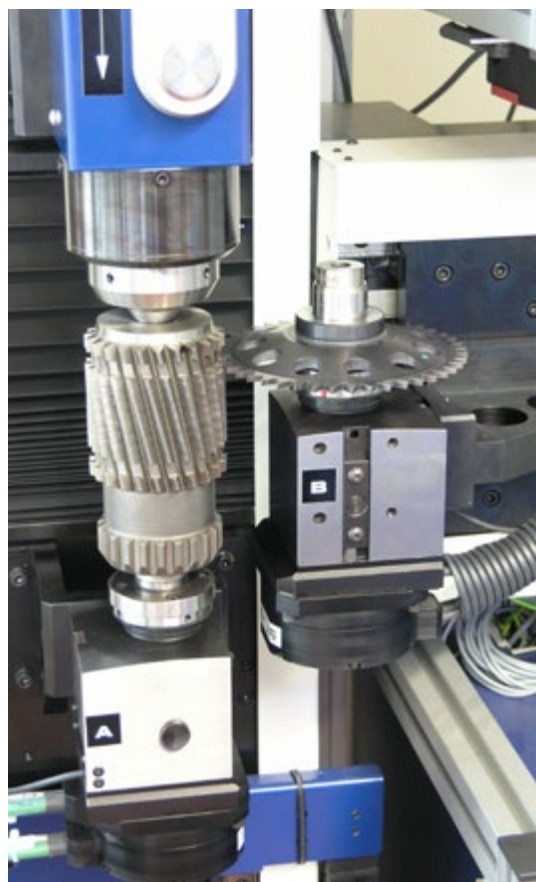
Gear flank analysing with disc roll master
