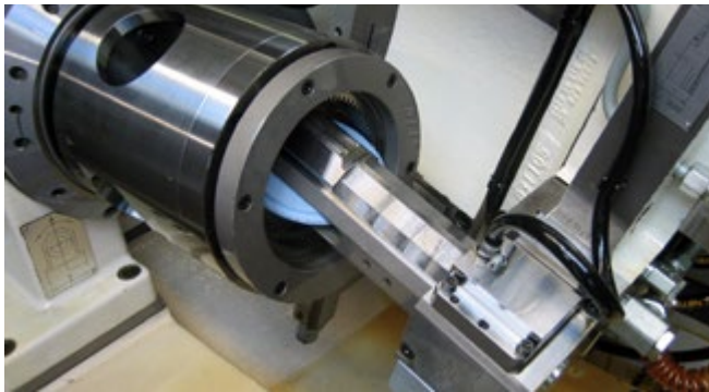
CNC grinding of internal profile
