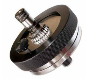
Frenco concentricity ring for runout checking.
