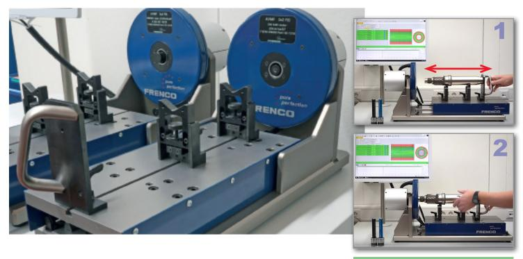
Inspect Internal & External Splines with the NEW Frenco **AVM 3X2 Horizontal Slide Bench Option with size over two balls measurement.** Check out this new development from Frenco Gmbh, world leader in spline metrology.
