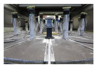
**APPLICATION:** Within one year, the original 10-ton blank was ground to its final convex aspherical shape with a thickness of only 10 cm and a final mass of 3 tons using Kostyrka® Adaptive Clamping at Schott AG in Mainz Germany.
