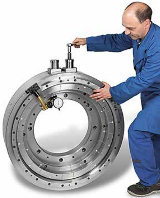
A MyTEC technician checks the runout of a large clamping tool.
