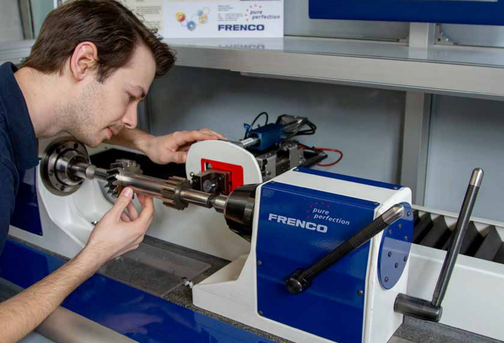
A Frenco tech works on the final assembly of a cluster shaft checker. (Photos courtesy: Euro-Tech)
